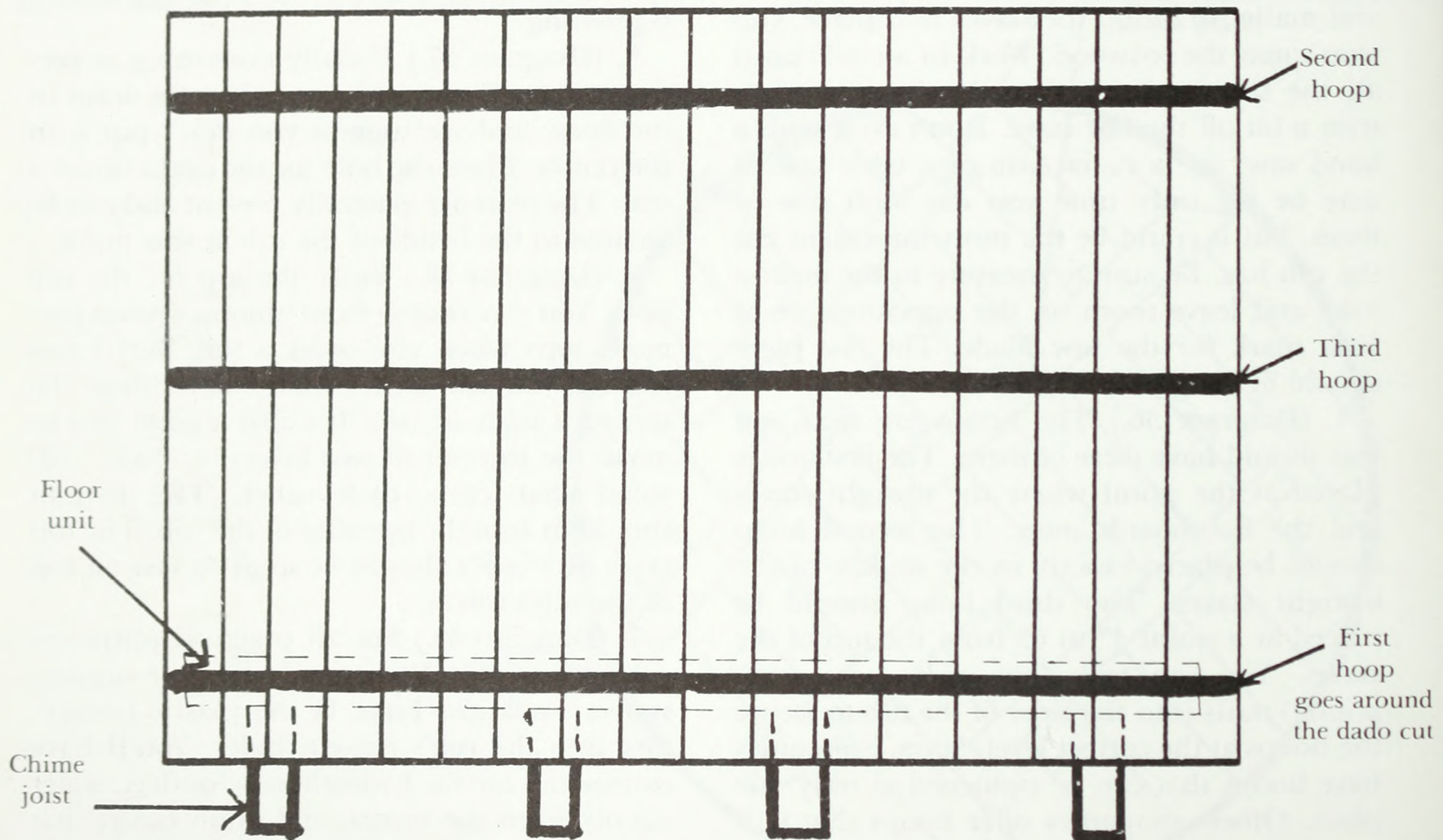
DIAGRAM 36. Step 4: Placement of steel hoops.
